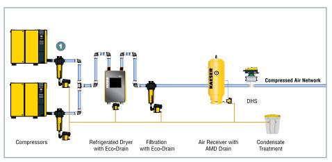
When the supply of air is the priority, the air main charging valve is set so that the default is "normally open". In case of power failure, the valve remains open, ensuring air supply. For systems which are shut down infrequently and have no leaks in the supply side piping, this field adjustable setting allows for any storage receiver after the air main charging valve to supplement air during start up conditions, further minimizing system exposure to high velocity air and faster start up.
