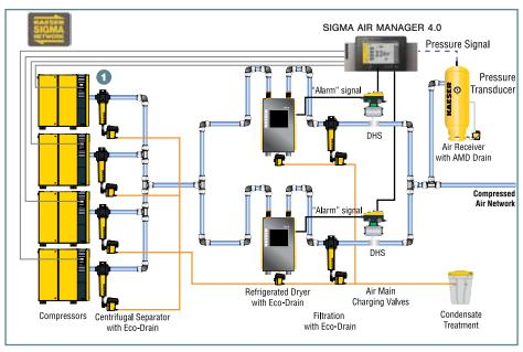
The second example shows a multiple compressor system with two parallel air treatment lines all controlled by a SIGMA AIR MANAGER<sup>®</sup> (SAM) 4.0. A standard feature of the DHS is its ability to connect to a SAM 4.0 by the KAESER SIGMA NETWORK. The SAM 4.0 can modify DHS 4.0 parameters and monitor for alarms. With optional inputs, the DHS can also close in case of a dryer failure or alarm.
