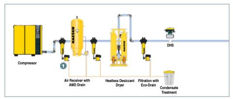
In its default configuration, the air main charging valve (DHS) is pre-set to close if the demand exceeds supply, pressure falls below the set point, or in case of power outage. It minimizes air velocity at start up and maintains air supply side pressure. For systems which are shut down frequently, this option further minimizes periods of high velocity air.
