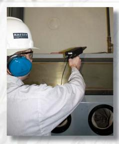
Kaeser uses the latest generation in ultrasonic leak detectors with onboard data logging. In addition to tagging your leaks, you will receive a detailed report with the location and approximate leak rate of each leak found. With this information, you can determine the best leak repair plan.
